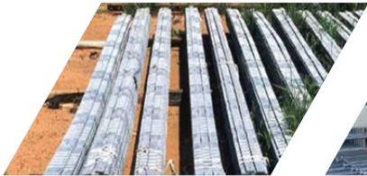
Steel strips reinforcement
